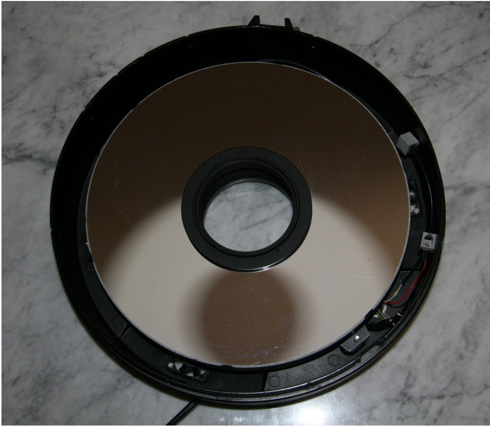
The primary installed, heating cable connected
