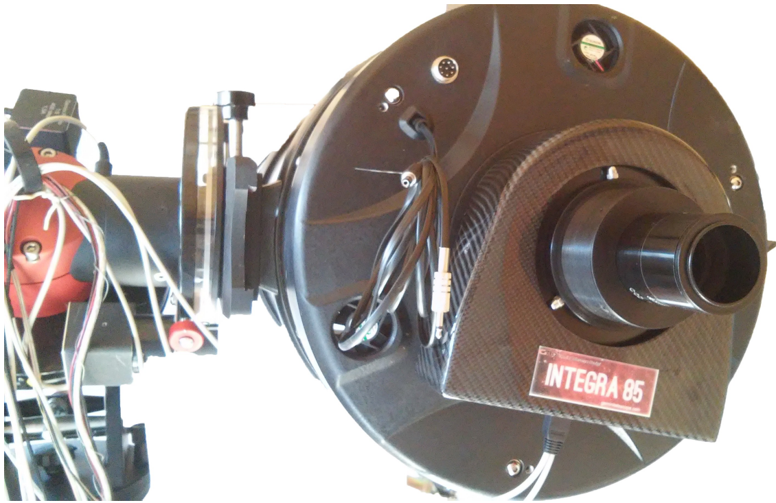
OTA on the mount, custom adapter attached to the Integra85
