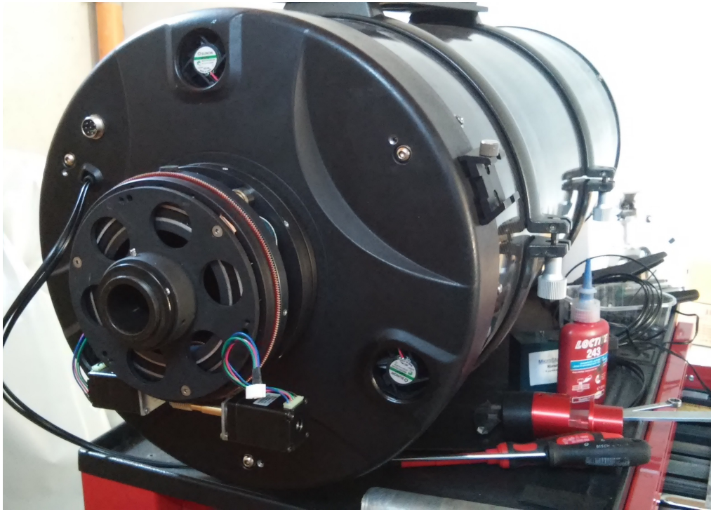
Integra 85 installed and collimated
