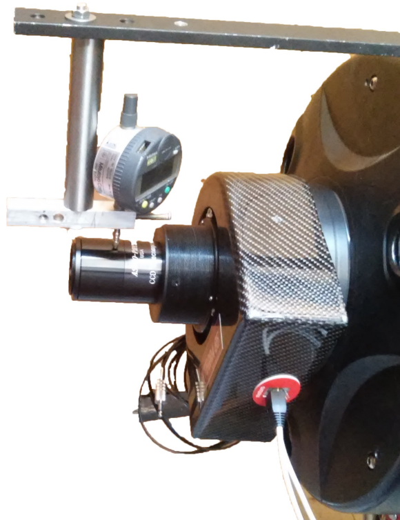
Rotator being collimated with a digital dial gauge
