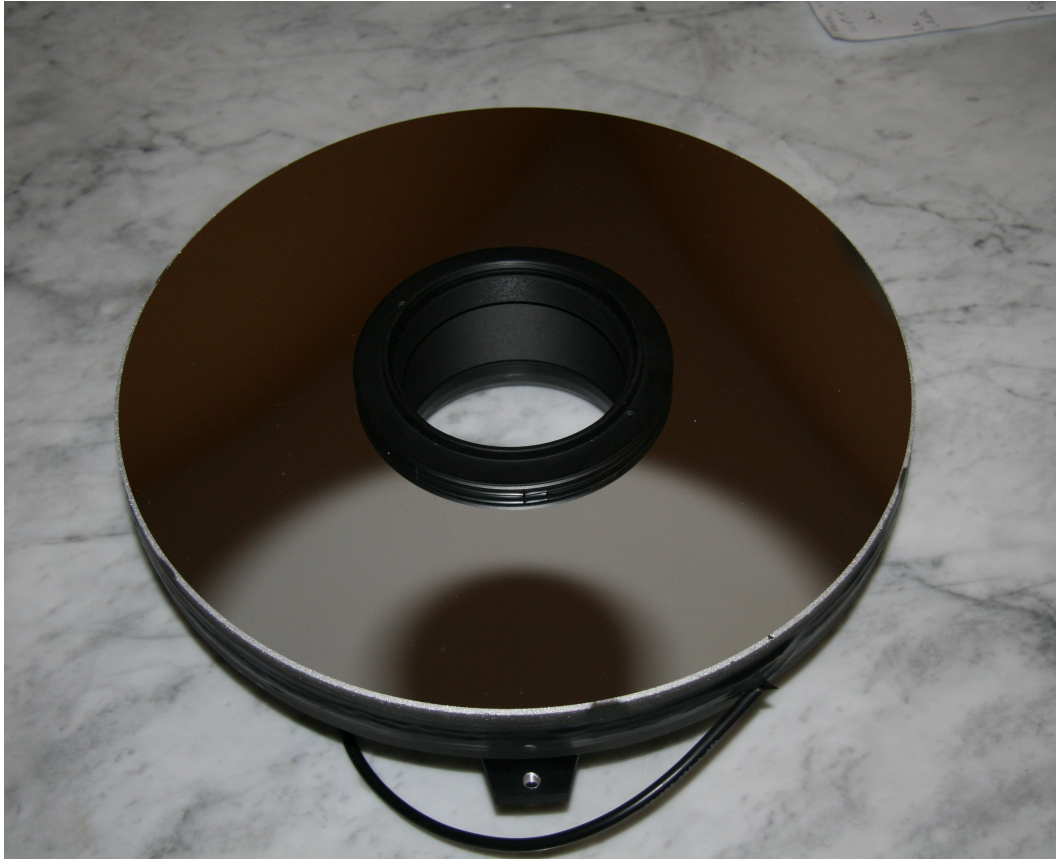
The primary mirror with the heating resistance installed
